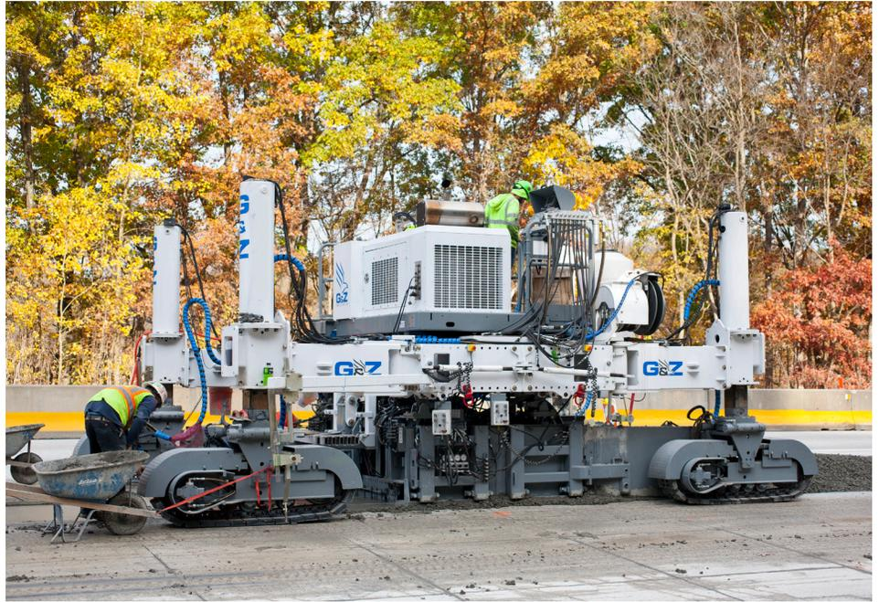
▲ The universal bolting pattern on the side of paver or bolster matches the bolting pattern on the center module of the tractor frame. This bolting pattern allows options such as stringless masts to be mounted per contractor preference as well as offset molds, conveyors, and other attachments to be mounted in a variety of ways to accommodate jobsite conditions.
