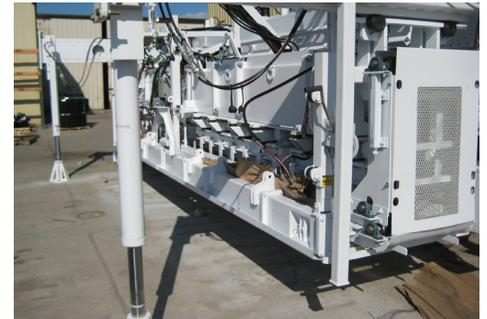
▲ With the use of the DBI Loading stands, the DBI can be loaded without the use of a crane.
