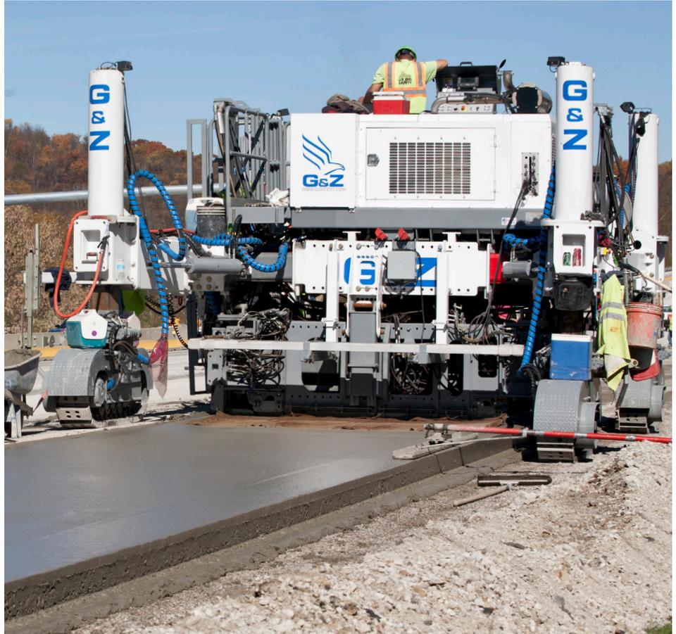
▲ AccuSteer and SmartLeg systems take paver productivity to the next level. The two systems work in tandem to adjust the swing leg angle on-the-fly while the crawler track automatically steers straight ahead. These two systems rapidly and semi-automatically reconfigure the machine into the transport configuration.
