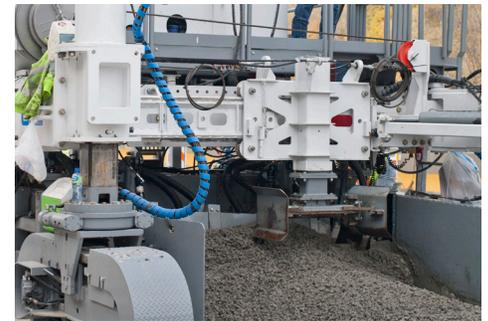
The powerful spreader plow spreads more concrete, faster and more economically than an auger, and it is easier to change width.
