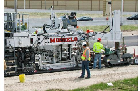
▲ The bolster extensions allow the S400 to continue to utilize its swing legs and maintain a narrow overall width for tight track line situations.
