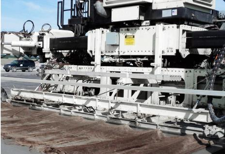
As an option, the S400 can be fitted with G&Z's proven Trailing Finishing Pan (TFP). The TFP provides a proven method of finishing the pavement surface and edges.
